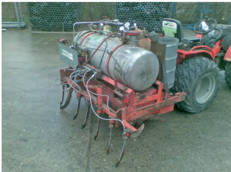
Fig. 2. Typical soil-disinfection machine.
