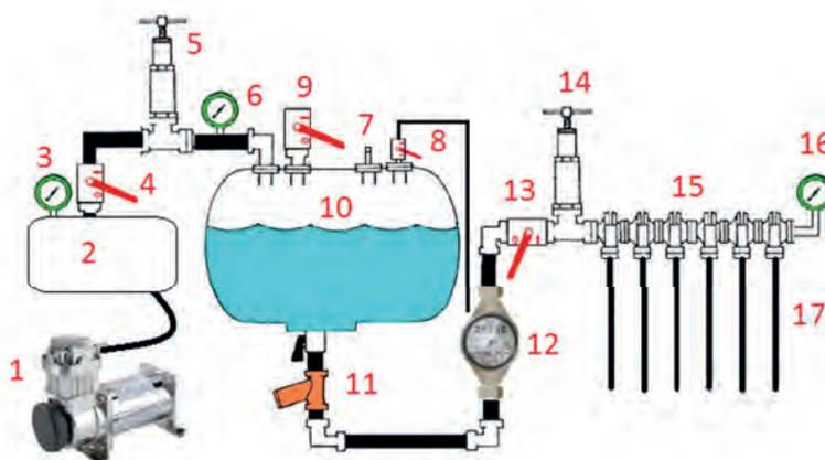
Fig. 3. Hydraulic scheme of a soil-disinfection machine.
