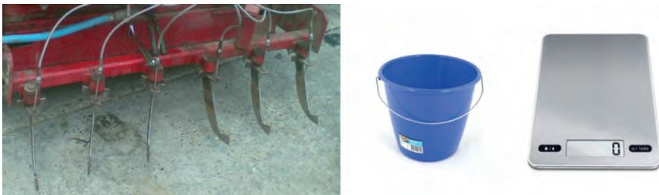
Fig. 4. Soil-disinfection machine injectors, pattern measurement.
