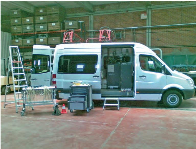
Fig. 1. Inspection van with test equipment.
