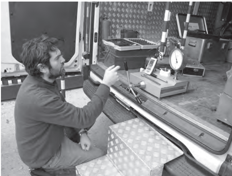
Fig. 1. The function test of a pressure gauge.
