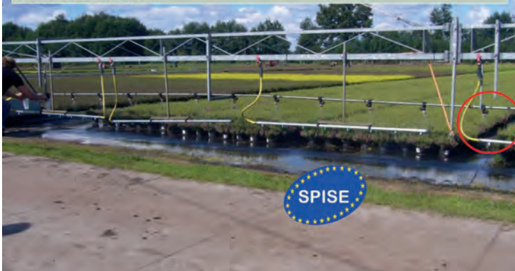
Fig. 2. Measuring the flow rates of single nozzles for evaluation of the cross distribution.
