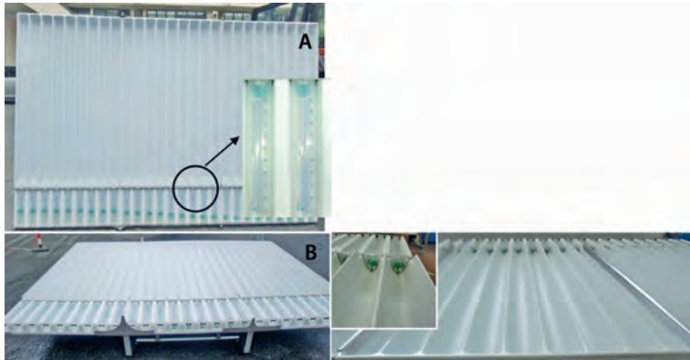
Fig. 3. Examples of manual horizontal patternator.
