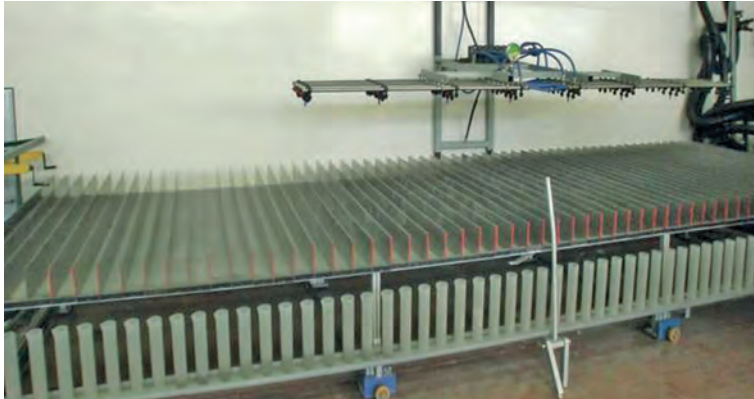
Fig. 3. Horizontal test bench complying with ISO 5682-1 standard used in the tests.
