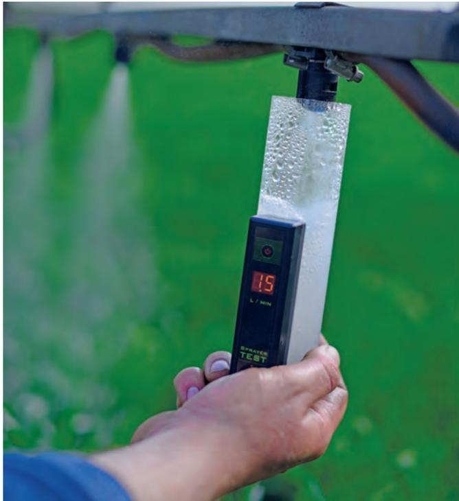
Fig. 2. SprayerTEST in use.
