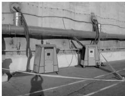
Fig. 7 picture of two ozone generators in action at a treatment of a large elevator Treating an entire structure is difficult; an alternative is to focus on the outlet silo semi continuous treatment.
