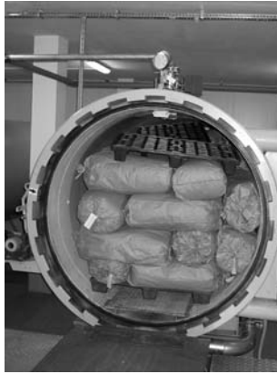
Fig. 7 high pressure chambers
