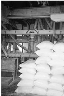
**Fig. 8** Funnel trap for stored-product moths in a mill
