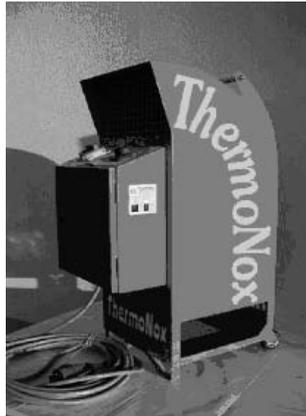
**Fig. 2** ThermoNox heater with 18.75 kW (0.75 kW for the fan)
