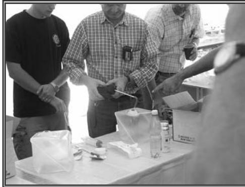
**Fig. 5** Phosphine resistance test kit.
