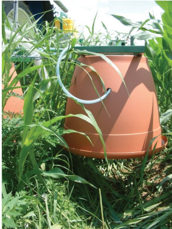
Figure 1. WeedSeeker sensor-sprayers shielded by plastic container
