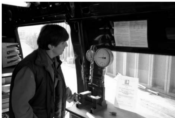
Fig. 5 Testing the work manometer
