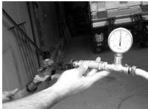
Fig. 2 Test bench to assess pressure drop for spray lances
