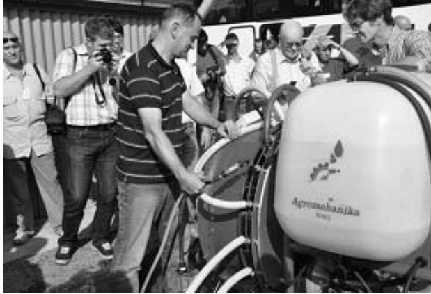
Fig. 4 Determination of the nozzle output of a vineyard sprayer at Hodonin
