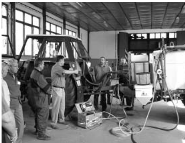
Fig. 3 Measuring of the pump capacity at Rovinka
