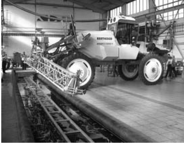
Fig. 2 Determination of the cross distribution by mobile spray scanner at Hustopeče
