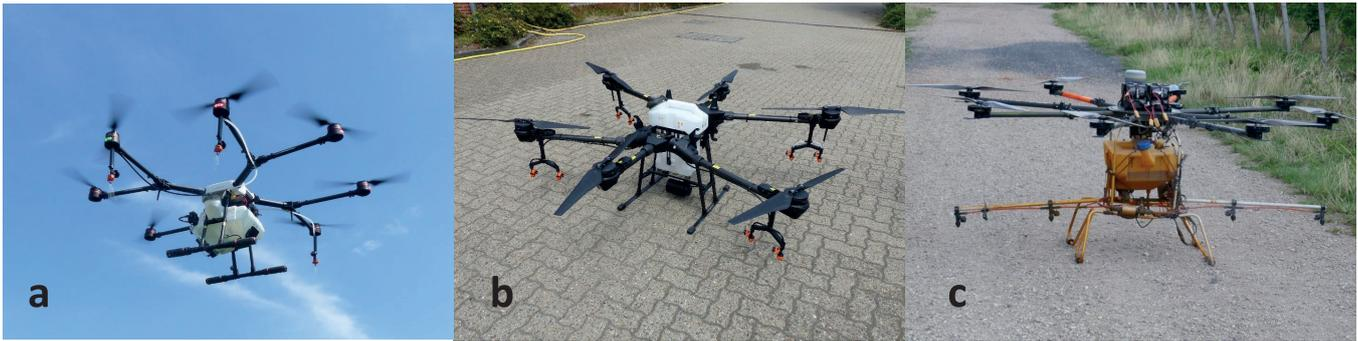
Fig. 1. Drones used for the experiments. a) DJI Agras MG-1 (max. take-off mass 24 kg, max. payload 10 kg), b) DJI Agras T16 (41 kg, 15 kg), c) Multikopter.de EVO-X8 (50 kg, 17 kg)
