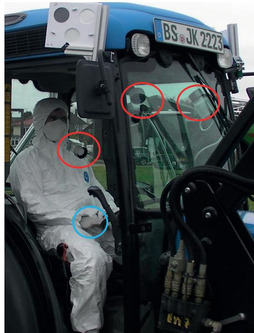
Fig. 4. The detectors and the placing of the detectors to measure exposure within the cabin
