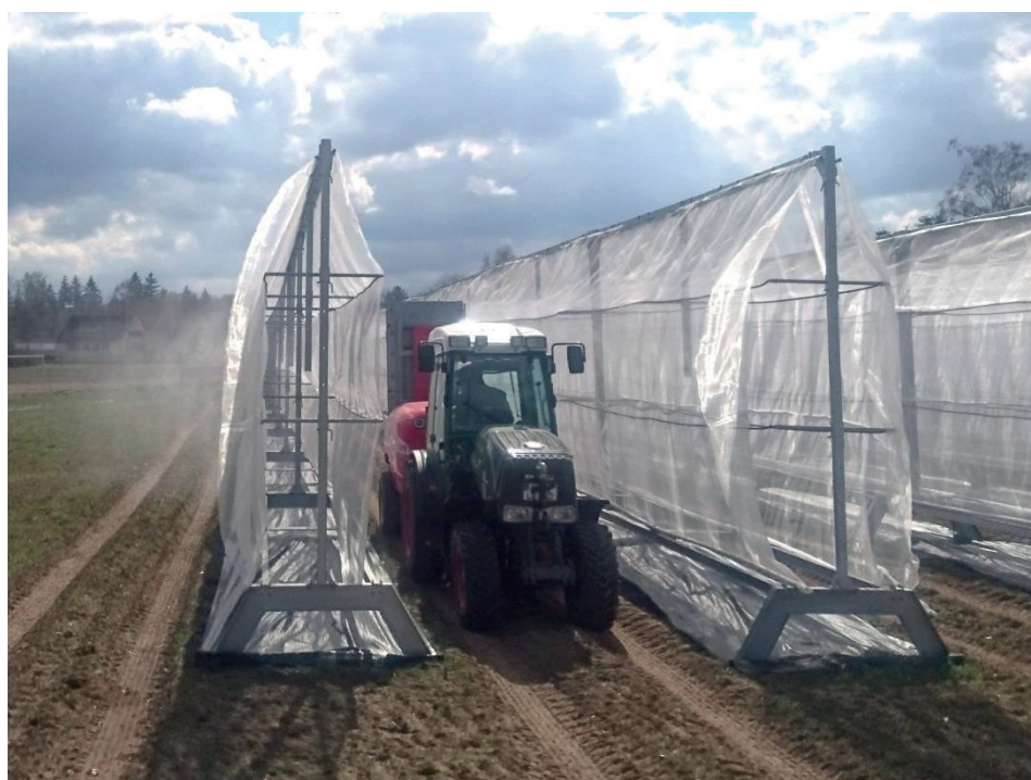
Fig. 1. Drift measurement in the model canopy with an air-assisted sprayer.
