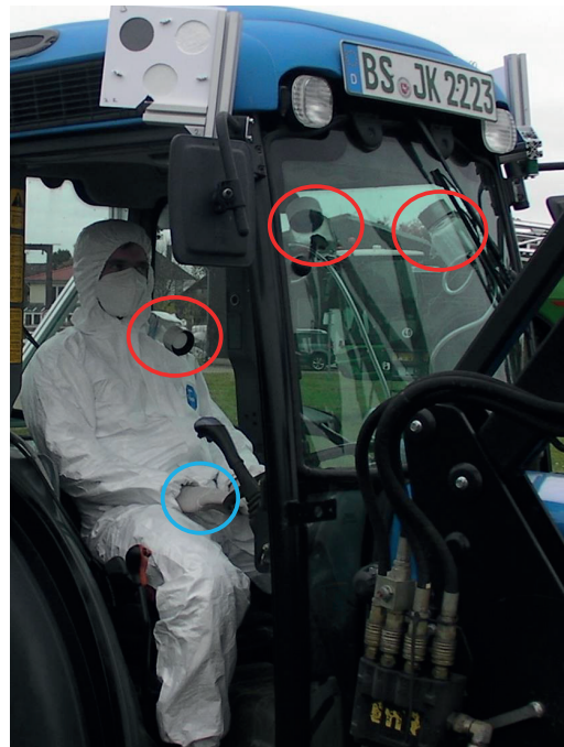
Fig. 4. The detectors and the placing of the detectors to measure exposure within the cabin
