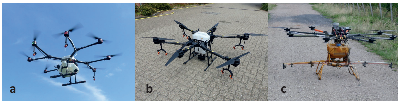
Fig. 1. Drones used for the experiments. a) DJI Agras MG-1 (max. take-off mass 24 kg, max. payload 10 kg), b) DJI Agras T16 (41 kg, 15 kg), c) Multikopter.de EVO-X8 (50 kg, 17 kg)
