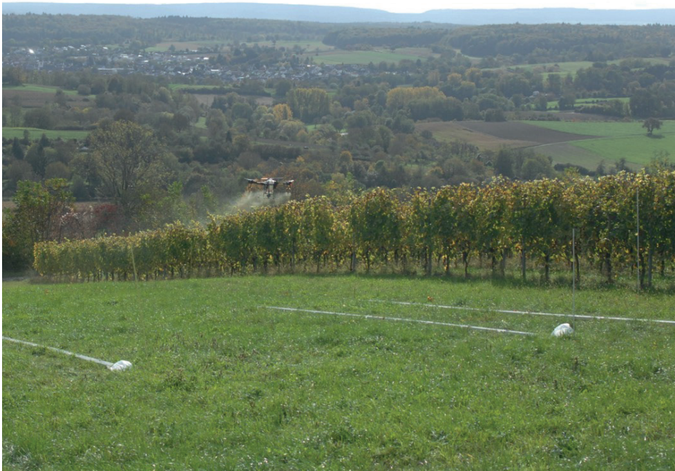
Fig. 3. View on the inclined vineyard in Weingarten during a test with the drone applying the test liquid, the short grass canopy on the downwind area and the planks supporting the petri dishes for drift sediment collection
