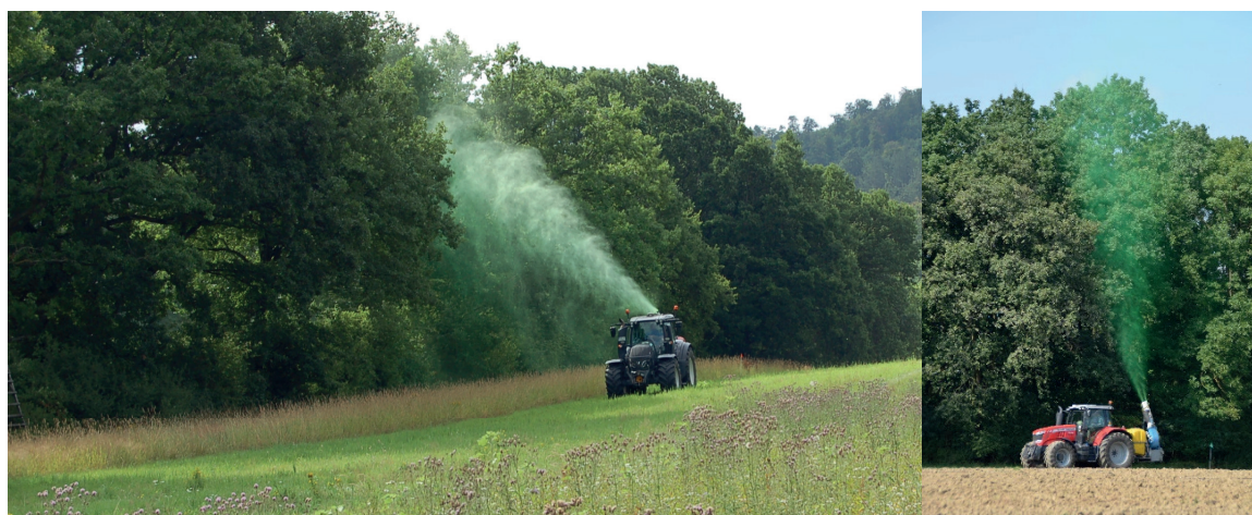
Fig. 4. Treatment of an avenue (left) and a forest edge (right) with a cannon sprayer.
