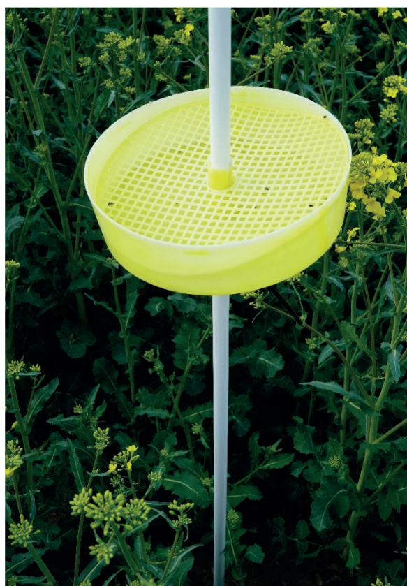
Fig. 2. Photographs of a yellow water trap (YWT) and a digital yellow water trap (DYWT) in an oilseed rape field. Note the solar power camera on top of the DYWT.
