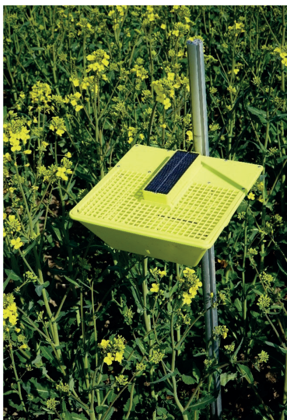
Fig. 2. Photographs of a yellow water trap (YWT) and a digital yellow water trap (DYWT) in an oilseed rape field. Note the solar power camera on top of the DYWT.
