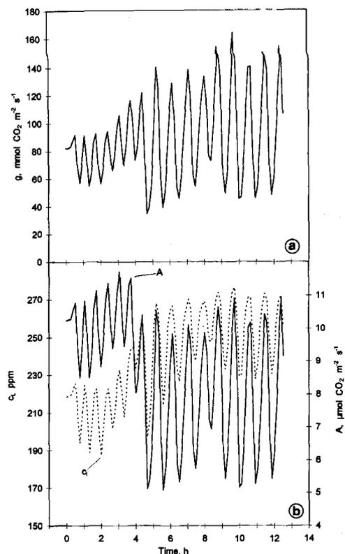
Fig. 2: Stomatal oscillations ( $g_{\text{CO}_2}$ ) at constant ambient conditions of the cuvette, determined by (a) gas exchange measurements leading to (b) synchronous alterations of intercellular  $\text{CO}_2$  concentration ( $c_i$ ) and photosynthesis (A).
