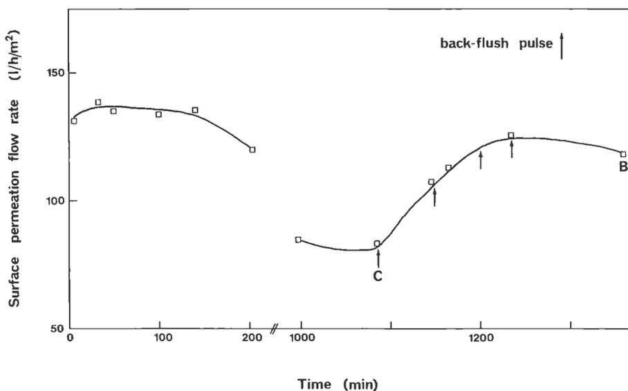
Fig. 1: Surface permeation flow rate ( $1 \text{ h}^{-1} \text{ m}^{-2}$ ) as a function of time of cross-flow microfiltration of a young red wine on a prototype mineral membrane (average pore size  $0.2 \mu\text{m}$ ). Samples of the wine permeate were withdrawn at times 18 h (2 min after the first back-flush pulse, sample C) and 22 h 40 min (sample B, final permeate).
