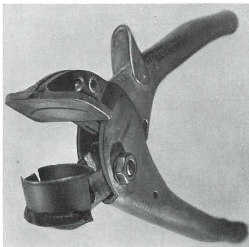
Fig. 1: Modified pair of anvil-type secateurs for the removal of single buds
